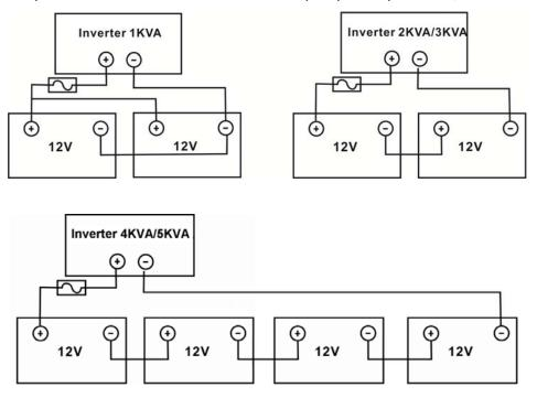
3. Insert the ring terminal of battery cable flatly into battery connector of inverter and make sure the bolts are tightened with torque of 2-3 Nm. Make sure polarity at both the battery and the inverter/charge is correctly connected and ring terminals are tightly screwed to the battery terminals.
