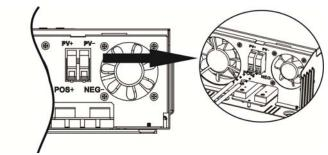
3. Make sure the wires are securely connected.
