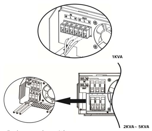
5. Make sure the wires are securely connected.
