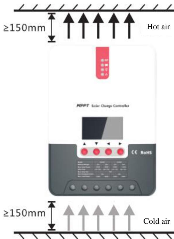
Fig. 2.1 Installation and heat dissipation
